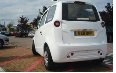
The new design features a bonded aluminium chassis built by Lotus, as well as Lithium battery pack, high temperature fuel cell, twin motors and onboard storage of I.8kg of hydrogen to give the fuel cell version a range of around I00 miles. With a view to delivering a fully EU Type Approved vehicle when in production, the H2EV has been through a range of simulated crash testing processes to validate the design.
