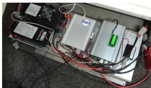
Figure 12 Microcab DC/DC component bay
