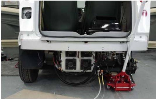
Figure 4: H2EV undergoing static test in Microcab, note the Horizon Stack and its location (centre), as well as the charging socket (upper left)
